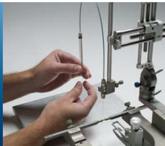
Many delicate neuroscience, stem cell and chemical dispensing applications require the use of pulled glass needles, also known as glass capillary needles, or PEEK tubing with precision syringes, as opposed to stainless steel needles. Properly attaching a pulled glass needle or a length of PEEK tubing to a syringe is difficult, and the traditional use of wax or other workarounds often exposes the experiment or technique to inaccuracy or contamination.
