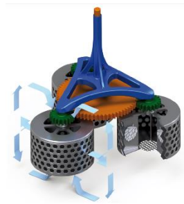
Fig. 2: Virtual 3D model of the Planetary Rotating Bed Reactors (PRBR) with a view of the reactor chamber and indicated flow pattern (Source: A Novel Dry Hopping Technology: Kinematic Modelling of a Planetary Rotating Bed Reactor )
